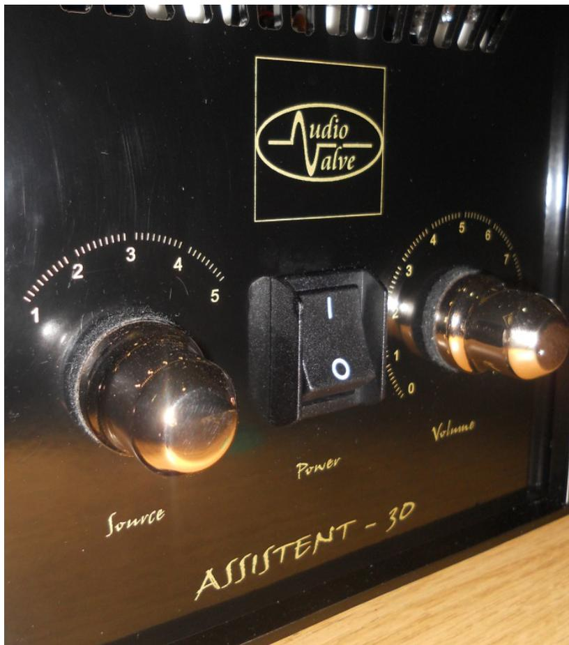
On the right side of the ASSISTENT 30 front panel is located the volume potentiometer by the 2 section ALPS potentiometer guaranteed a high accurate analog volume control .
